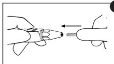
1. With thumb nut loosened, insert new Sani-Tip® disposable tip and push into adapter as far as possible. While still pushing inward, twist tip 1/2 turn clockwise to create a watertight seal over internal tapered water spindle.
