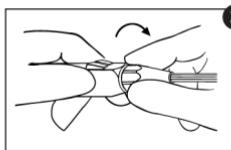
2. Hand tighten thumb nut. To redirect tip, push in on tip while rotating clockwise.
